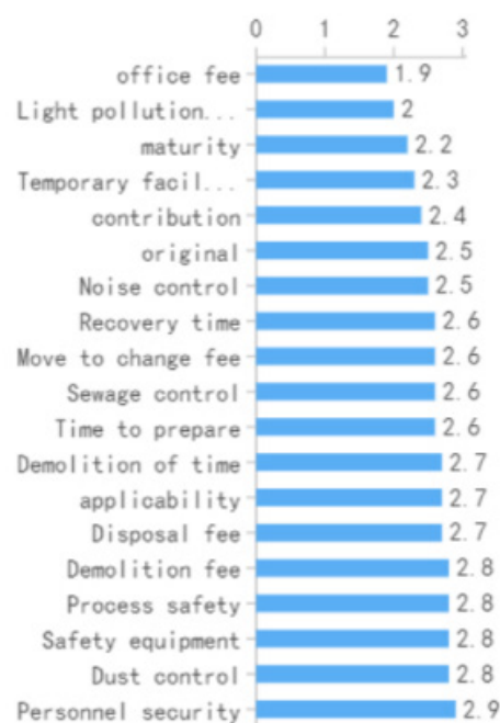
Figure. 1. Factors affecting the selection of urban overpass demolition scheme
